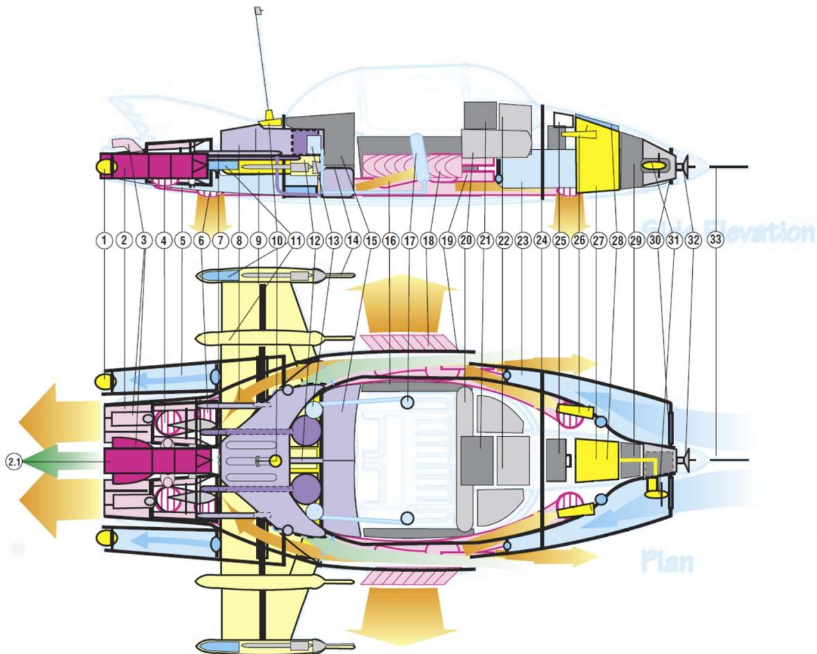
1. **Rear Navigation Lights** (2) Port & Starboard, with rear ballast eject through valve surround.
