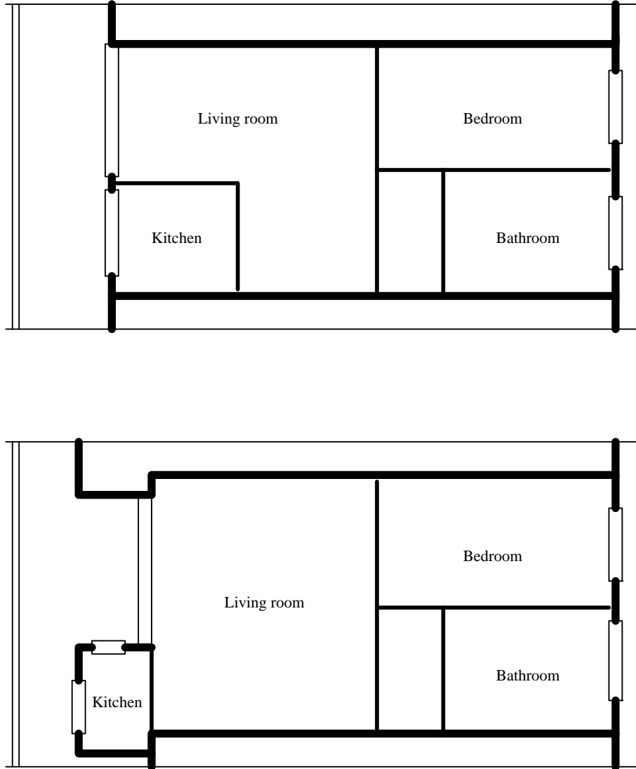
Figure 2: Proposed designs for single-bedroom deck-access flats (a) with a rectangular floorplan (b) with one flat overlapping the next
