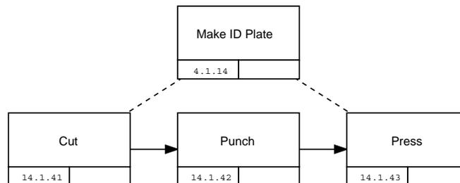
Figure 25: Process for manufacturing the 350-ID Plate
