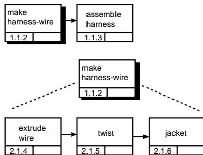
Figure 10: Production steps in the wire and cable department
