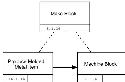
Figure 27: Process for manufacturing the 350-Block
