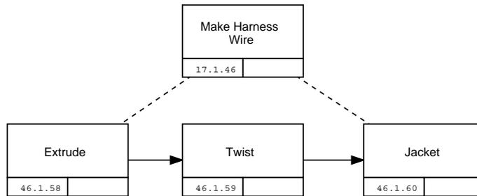
Figure 29: Process for manufacturing the 350-Wire
