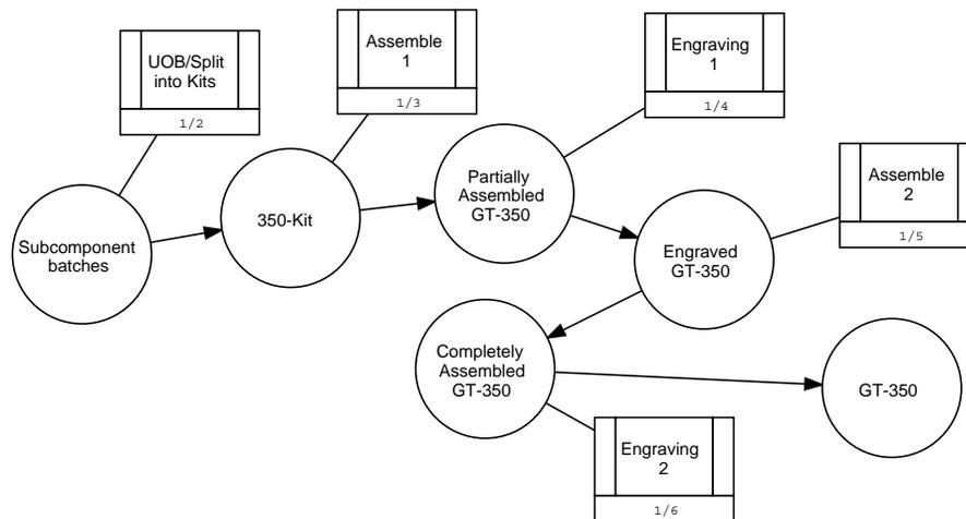
Figure 18: Object state transitions in the assembly department
