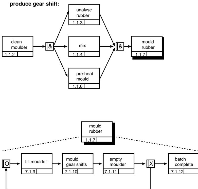
Figure 4: Production steps in the rubber works
