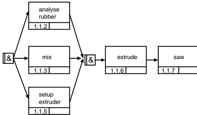
Figure 3: Production steps in the rubber works
