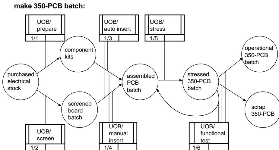
Figure 14: Object state transitions in the Electronics department
