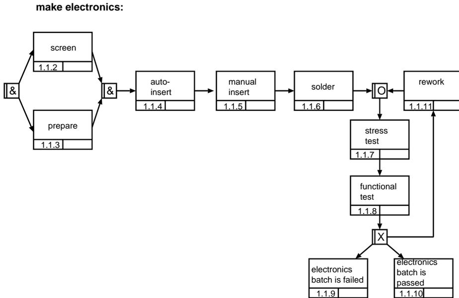
Figure 13: Production steps in the Electronics department
