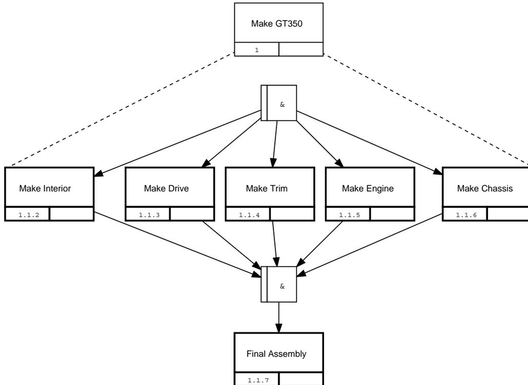
Figure 19: Top level process for manufacturing a GT-350
