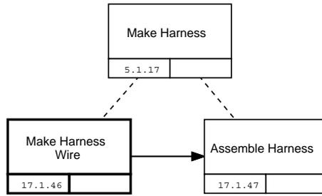
Figure 28: Process for manufacturing the 350-Harness
