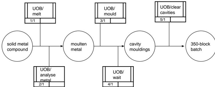
Figure 2: Object state transitions in the foundry
