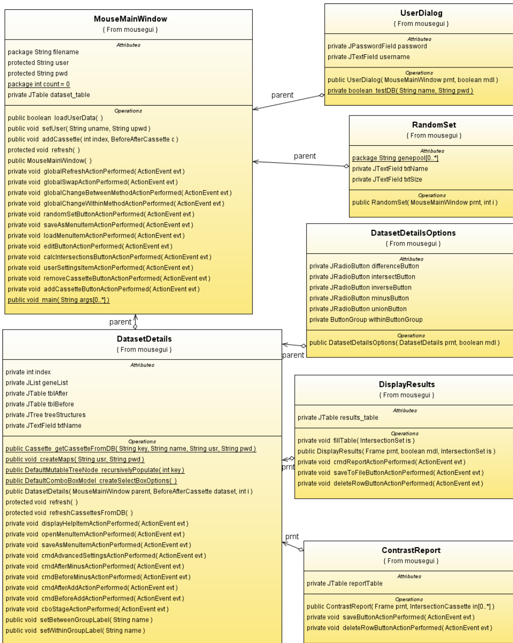
Figure A.2: Simplified UML Class Diagram of the MouseGui package.
