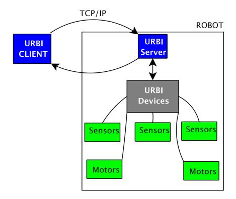
Figure 2.2: The URBI Client/Server Architecture
