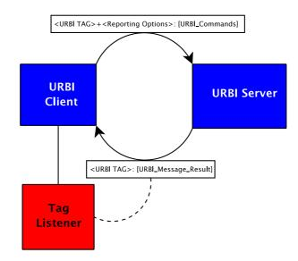
Figure 2.3: Using the Listener with URBI Tags. The dotted lines shows and indirect relationship between the tag and a registered URBI listener. The solid line indicates that the Listener is part of the URBI Client while the arrows represent the flow of data between the client and the server.
