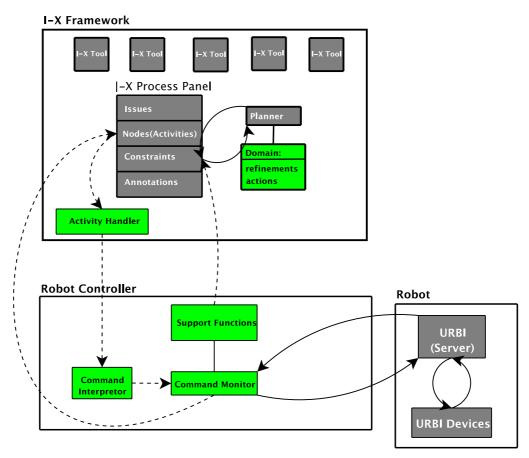
Figure 3.1: The Architectural Design of the project.
