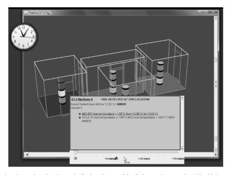
Fig. 8. At a later time, the user has selected more details about the state of the 'fire' room: the current hazard level is "now amber", due to the combination of belief and rule shown. Moreover the traffic light (and the time slider) indicate that there is a future "red" hazard level predicted (for approximately 6 minutes into the future).
