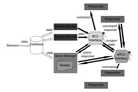
Fig. 1. The FireGrid system architecture from a C2 perspective. Arrows show principal communication flows only, with inter-agent communications indicated by solid arrows.
