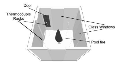
Fig. 2. Layout of smoke-box with instrumentation.
