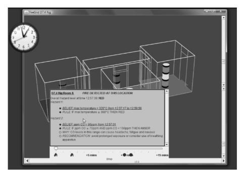
Fig. 9. At a still later time, the hazard level is now "red" (and has deteriorated in the other locations), and the presence of multiple hazards is indicated by the rules. Note the explanation and recommendations attached to one of the rules.
