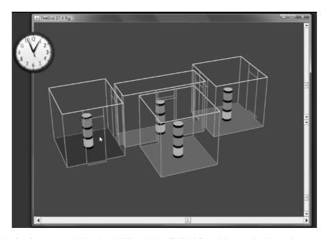
Fig. 7. C3I tool interface for 4-room (and 4-location) building, with "traffic light" for each location: in this case the green traffic lights indicate that fire-fighters can operate in every location; however, the red floor in the room under the cursor indicates that a fire has been detected there.
