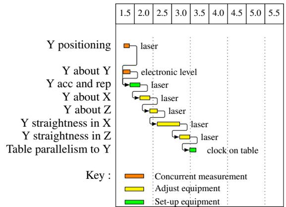
Figure 2: Excerpt from a produced calibration plan from the machine tool calibration application
