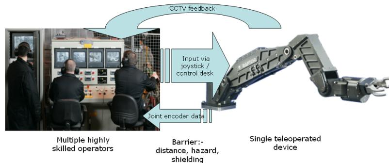
Figure 1 (multiple in the loop operators : single device)
