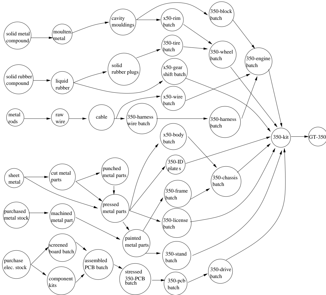
Figure 35: Flow of materials for production of the GT-350
