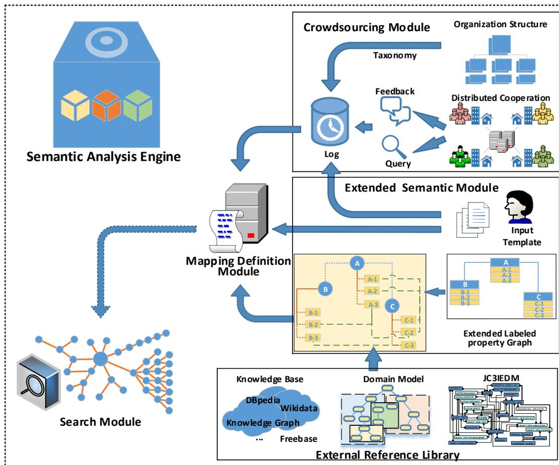
**Fig.5 Semantic analysis engine architecture**
