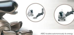
station when its energy is dropping. The pattern on the Energy Station Pole helps AIBO to localise and position itself quickly.
